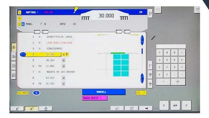
with 8.5"colordisplay and Touch-Screen operation for all standard cutting work
